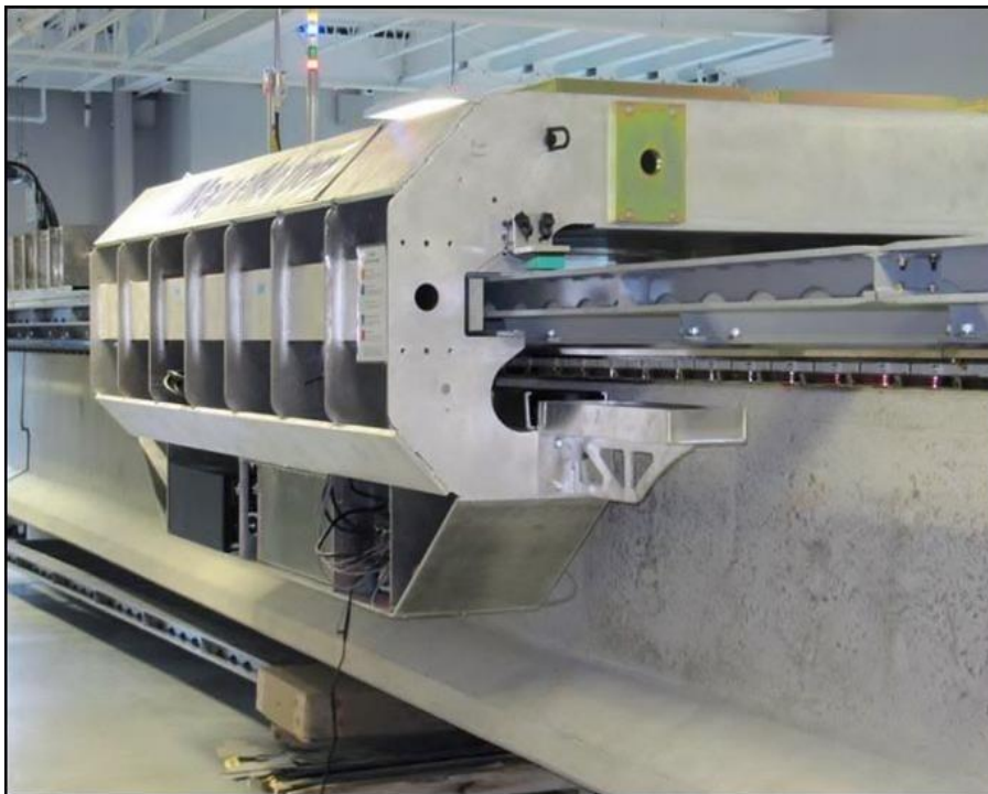
Figure 2b. The M3 test sled at MMI in Devens, Massachusetts. This test sled is capable of carrying a payload equivalent of a vehicle body and 18 to 20 passengers.
